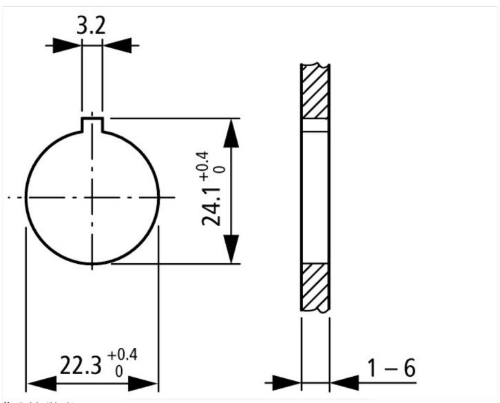
Mounting hole with lug slot
