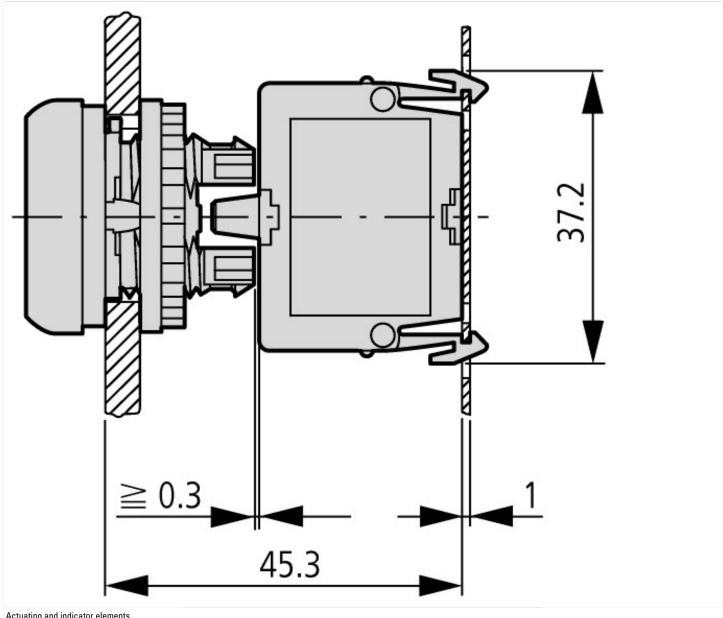
Actuating and indicator elements Base fixing
