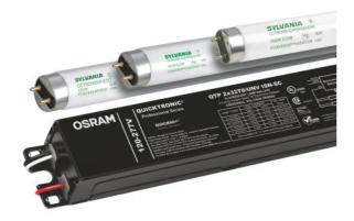
A QUICKTRONIC SYSTEM 32 UNV electronic T8 ballasts offer several advantages:— Operate OCTRON T8 lamps with maximum efficacy and high lumen output— 30-40% energy savings when compared to F40T12 magnetically ballasted systems— Parallel Circuitry: keeps remaining lamps lit if one or more go out3. Small Can Enclosure for:—low profile fixture design, transportation, inventory and ergonomic benefits
