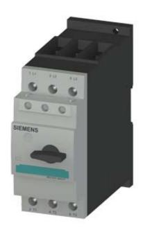
CIRCUIT-BREAKER SIZE S2, MOTOR PROTECTION CLASS 10 A-RELEASE 22...32A, N-RELEASE 416A SCREW CONNECTION W. INTEGRATED AUXILIARY SWITCH
